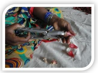
13.58± 1.012 mm. The developed Roselle calyces detacher is shown in Plate 1. A special stainless steel (SS -304) cutting blades made for the purpose of
